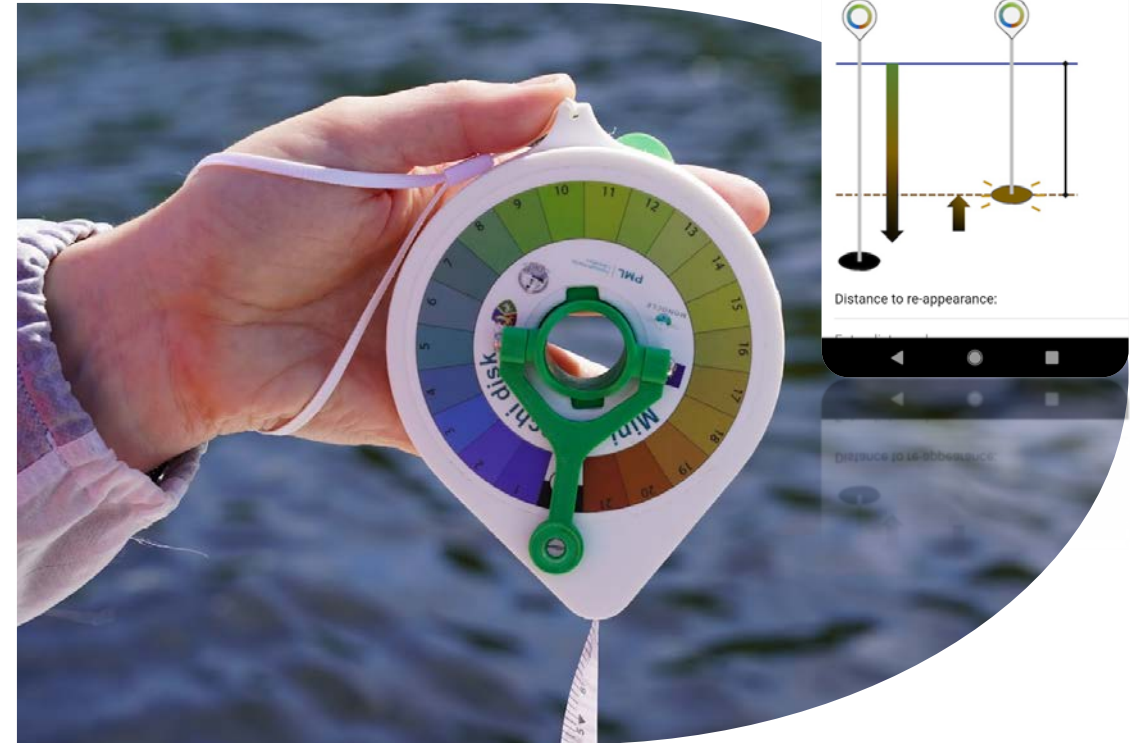
Mini-Secchi disk: transparency, colour-by-eye, pH 'mini Secchi' in app stores
