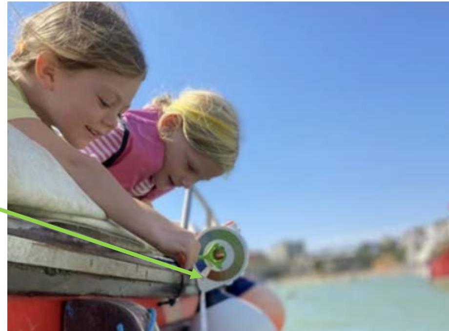
A mini-Secchi disk with FU scale
